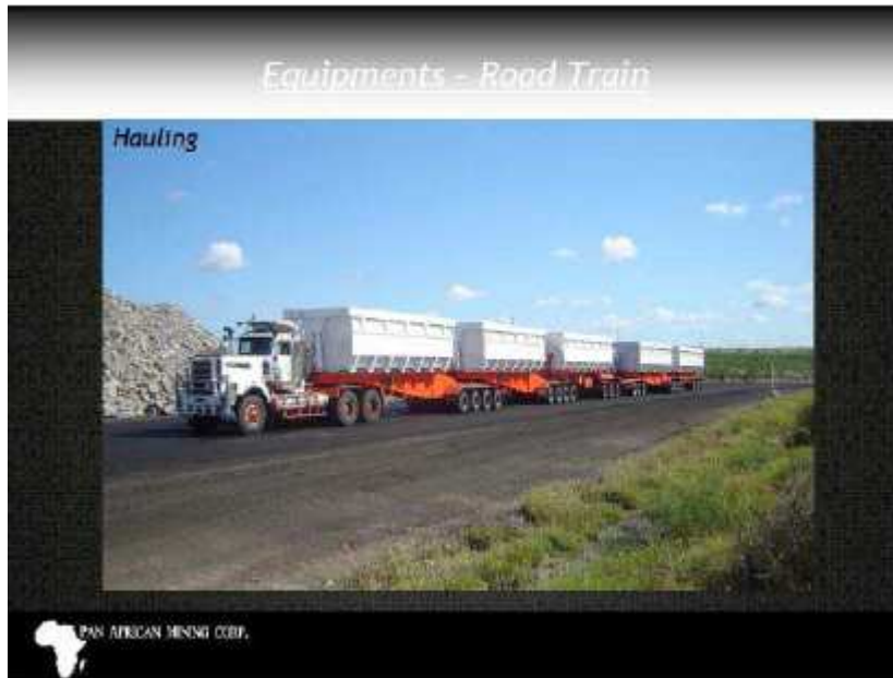
Planned traffic : A quad haul train : axel load of 13 T . Total DWT of 200 T . 200 Quad road train per day on one way consistent with 240.000 T / Week .
